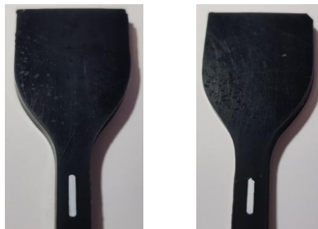
Figure 7: Well defined dash (left) and unsuitable dash (right)
